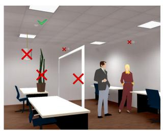
In order to improve the **Motion Detection**, it must be considered the higher sensitivity to tangential movements. Movements with axial direction to the sensor are detected worse than tangential ones.
