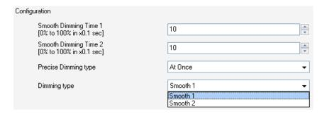
Smooth Dimming Times 1 and 2: this is the time LUMENTO X4 takes to perform soft luminosity transitions on the particular channel. There are two possible smooth transitions (Smooth 1 and Smooth 2). The times here refer to the complete transition, from 0% to 100%, and the permitted values are from 3 to 65535 tenths of a second. Both values are initially 10 (0.1 seconds), by default.
