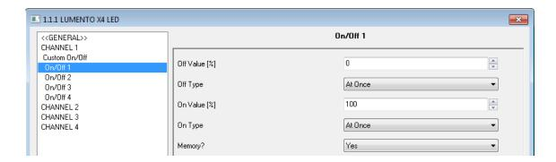
Figure 7. Custom ON/OFF configuration
