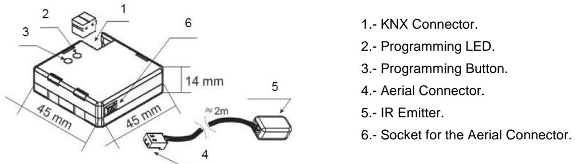
Figure 2. Element Diagram
