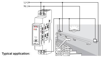
The staircase lighting time delay switch ASM-01/U operating the staircase lighting works in 3-wire installation. Push-buttons (equipped with illumination) can be connected parallely.
