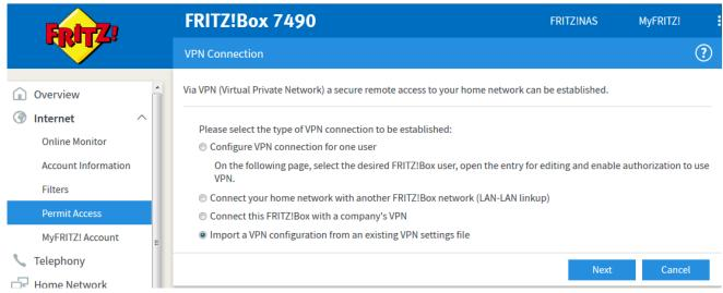
Figure 17: Fritzbox VPN-Server – choose means of configuration
