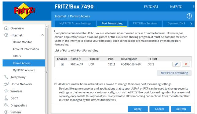
Figure 3: Settings in the DSL router (list of port forwarding's)
