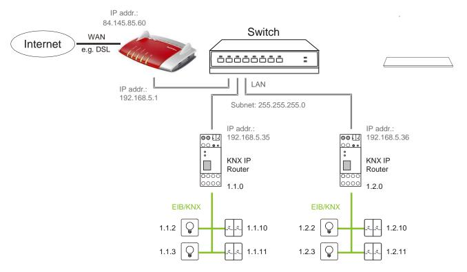
Figure 1: KNX installation
