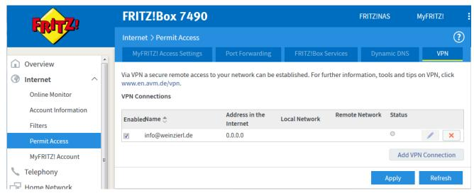
Figure 19: Fritzbox VPN-Server – opening the VPN connection
