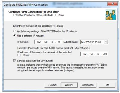
Figure 11: Subnet definition of LAN in building B
