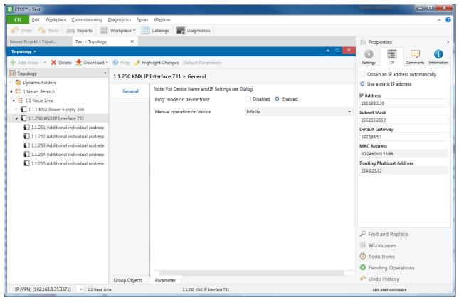
Figure 4: IP configuration (part 1)
