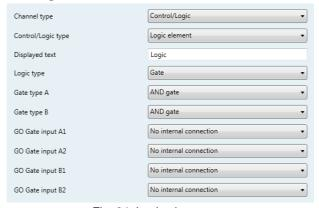
Fig. 24: Logic element
