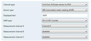
Abb. 15: Automated meter reading
