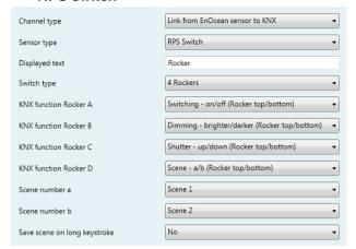
Fig. 6: RPS switch (sensor)
