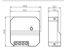
Flush-mounted RF KNX actuators
