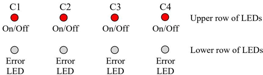
The device dims down to 0 % in the event of excess temperature or a short circuit in the load, and the lower LED flashes.
