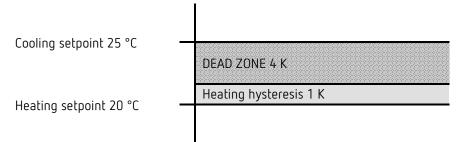
The dead zone (4 K) is increased by the value of the hysteresis (1K) and offsets the cooling set point value to 25  $^{\circ}$ C.
