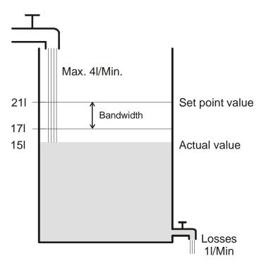
If the filling quantity is 15 I, there is a control deviation of 21 I - 15 I = 6 IAs our actual value lies outside the bandwidth, the control will operate the feed at 100%, i.e. with 4 I/minute.
