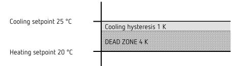
The dead zone (4 K) is increased by the value of the hysteresis (1K) and offsets the cooling set point value to 25  $^{\circ}$ C.
