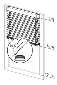
Step 2: Height running time = 24 s, upwards direction (Difference between current position 50 % and new position 30 % = 20 % of height running time) plus
