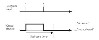
without manual OFF: A telegram with the object value "0" has no effects. The staircase timer set continues to run normally until the end. An OFF delay cannot be set.
