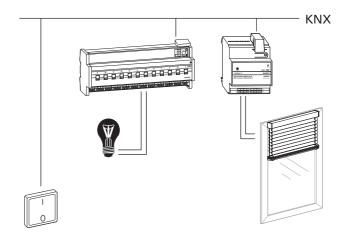
The preset function allows you, for example, to switch on the lighting and move the roller shutter at the same time by pressing one push-button. If you enter the value 0 % (roller shutter open) for preset function 1 and the value 100 % (roller shutter closed) for preset value 2, then pressing one push-button gives you the following control:
