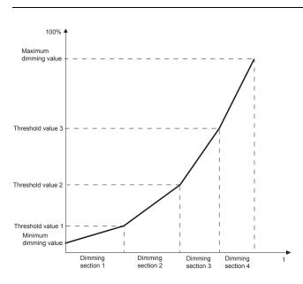
The dimming hardware requires at least 500 ms to run through the entire dimming range from 0% to 100%. Please observe this limit value when setting the dimming times for the individual dimming sections. Overall dimming times which are shorter than 500 ms cannot be executed by the hardware.
