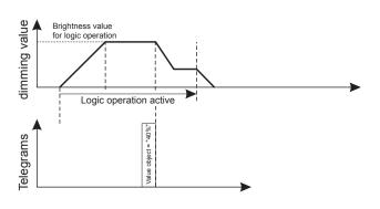
The brightness of the logic operation result and the dimming speed is defined by the last telegram.
