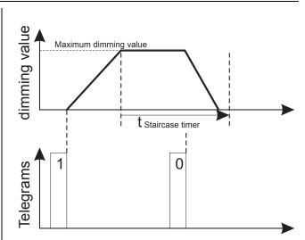
If an OFF delay has been parameterised, this function is now active and the output only switches off after the delay time has expired.
