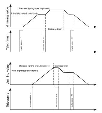
You can use this, for example, for temporary continuous light switching (cleaning lighting). An ON telegram from the switch object causes the light in the staircase lighting function to remain switched on continuously. Value, dimming, scene and central telegrams continue to be influential, however. For an application of this type, an initial brightness of 100% would be suitable when switching on.
