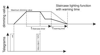
If you have parameterised a cut-out delay for the dimmer output, the warning time begins after the delay period has expired.
