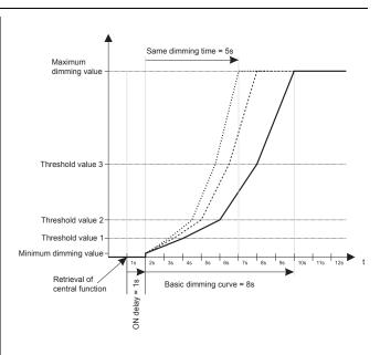
The ON delay is also retained with an identical dimming time. The dimming curve is compressed or extended in such a way that the dimming value is reached after the same dimming time. In other words, the calculation of the new dimming curve takes into account the pure dimming time (the same dimming time minus ON delay time).
