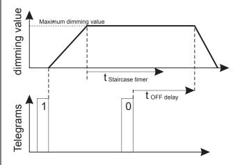
If you have selected the parameter value "without manual OFF", the staircase lighting function is not interrupted when a telegram with the value "0" is received, but continues to run normally until the staircase lighting time has expired.
