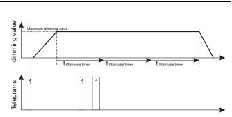
You can limit the potential running time using the "Max. number of time accumulations" parameter.
