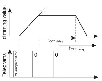
If the output receives a new telegram while an OFF delay is active, which creates an ON status, the OFF procedure is halted and the new set value is set.
