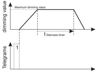
You can activate the staircase lighting function for each channel via a parameter:
