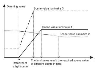
The "Same dimming time" function can be used to synchronise the different dimming times of the channels in such a way that all channels reach their set value at the same time. Using the "Time factor modifiable via the bus" parameter (via the communication object "Factor same dimming time"), the dimming times can also be synchronised for several dimming actuators.
