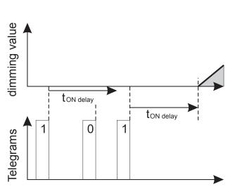
You can use a parameter to set whether the output channel remains switched off during the ON delay, or whether it is already set to the minimum dimming value.
