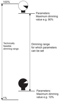
The dimming range which can be parameterised is set using the following parameters:
