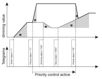
Parameter settings for the example in the image: - Behaviour at start of priority control "on" = "switch on to variable brightness" - Required brightness at start of priority control "off" in %~=~100
