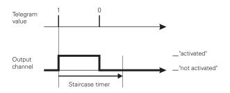
without manual OFF: A telegram with the object value "0" has no effect. The staircase timer set continues to run normally until the end. An OFF delay cannot be set.
