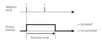
retriggerable: After a new telegram has been received with the object value "1", the staircase timer is restarted.
