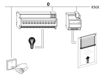
In this case, due to the fact that the roller shutter requires a certain running time to open, the light needs to be swiched off with a switch-off delay so that it doesn't suddenly become dark prematurely.
