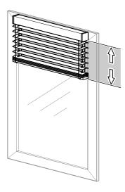
When the limit function is active, the drive only moves between the limit values. The limit applies for all movement commands from manual operation, automatic functions, scenes, presets and for movements from functions of lower priority.
