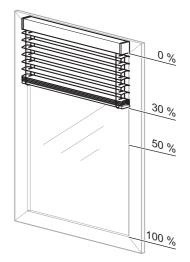
Step 3: Slat adjustment into the operating position after upwards movement = 1.25 s(Slat running time from 0 % to 50 %)
