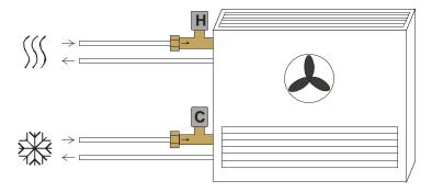
When used in a 4-pipe heating/cooling system the heating valve is connected to the V1 terminals and the cooling valve to the V2 terminals.
