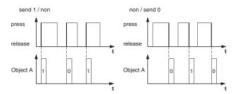
Object A = 1 Byte variable 0-255 value 1 = 255 value 2 = 50 action at pressed/released
