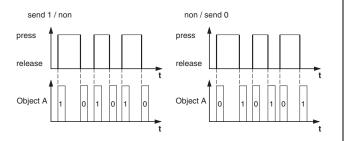
Object A = 1 Bit action at pressed/released
