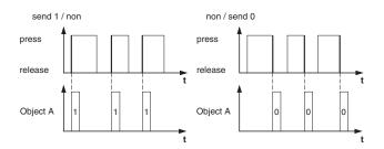
Object A = 1 Bit action at pressed/released
