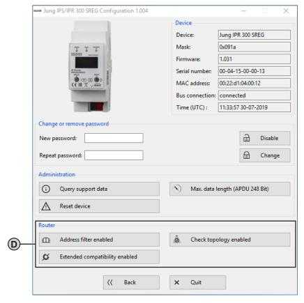
Fig. 21: Device configuration - IP router
