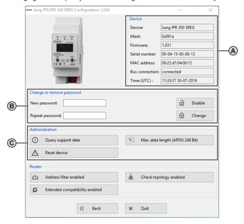
Fig. 20: Device configuration - IP router and IP interface
