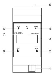
Fig. 1: Device components
