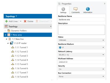
Fig. 5: Topology (left) and properties of the backbone
