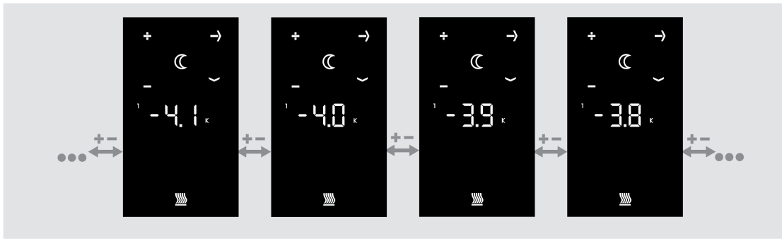
Figure 23: Setting the setpoint temperature "Lowering for night mode, heating"
