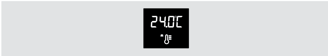
Figure 15: Indication of setpoint temperature
