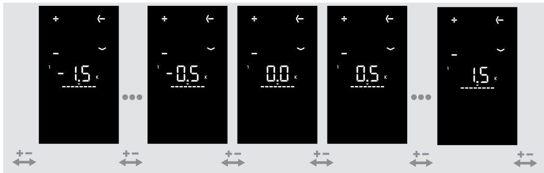
Figure 26: Setting the setpoint shift
