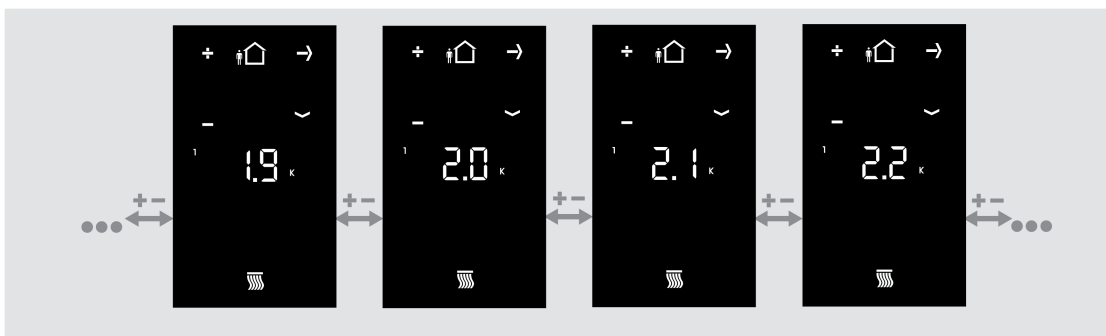
Figure 22: Setting the setpoint temperature "Raising for standby mode, cooling"
