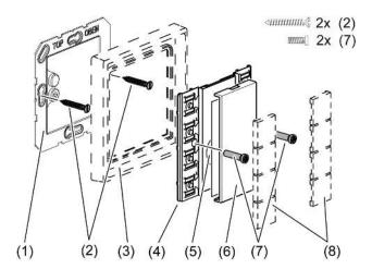
Figure 1: 4-gang radio wall transmitter module
