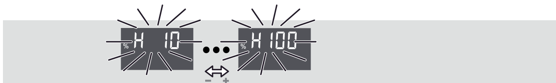
Figure 24: Setting the display brightness
