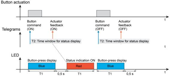
Figure 12: Example of a status display with the operating function "Switching" Telegram on pressing the button
