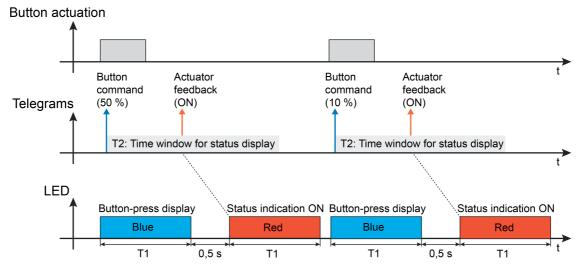
Figure 19: Example of a status display with the operating function "Value transmitter 1-byte" Telegram on pressing the button
