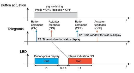
Figure 6: Example of a two-level actuation and status display for actuator feedback New time window for status display through multiple operating telegrams
