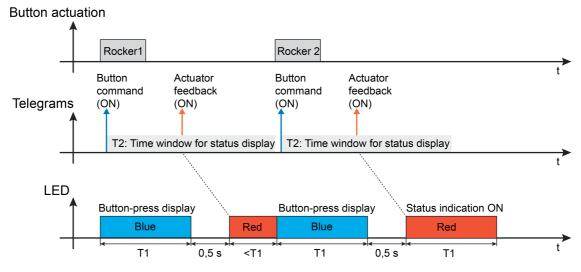
Figure 10: Example of a two-level actuation and status display Interruption of the display function through new button actuation
