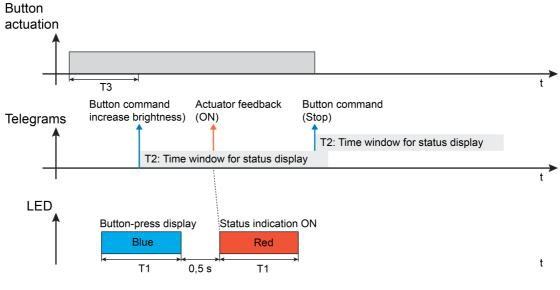
Figure 15: Example of a status display with the operating function "Dimming" with a long button-press
