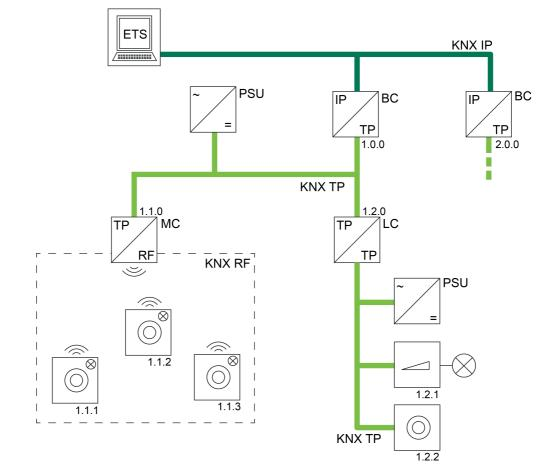
Figure 43: Example of a possible KNX topology with one KNX IP connection of the ETS (KNXnet/IP)
