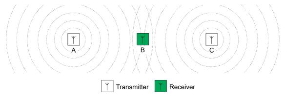
Figure 23: Radio collisions on the receiver due to the transmitter being too far away
