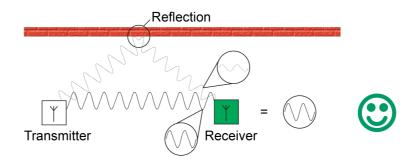
Figure 30: Interference has no effect on the receiver
