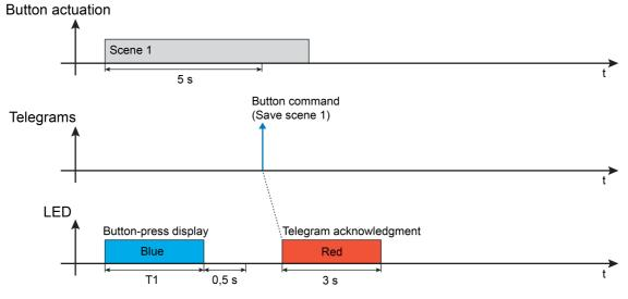
Figure 22: Example of an LED display with the operating function "Scene extension" Scene extension with memory function and telegram acknowledgement
