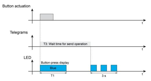
Figure 11: LED display in the case of a transmission error
