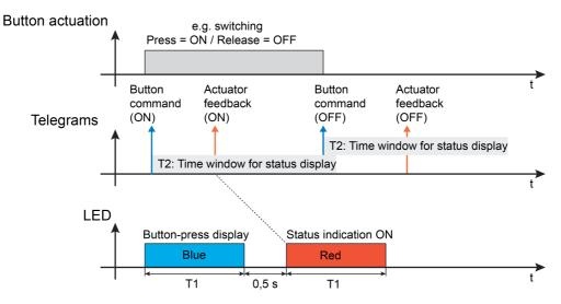
Figure 13: Example of a status display with the operating function "Switching" Telegram on pressing and releasing the button
