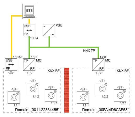
Figure 40: Example of a possible KNX topology with two RF lines and coupling via a TP main line (example)
