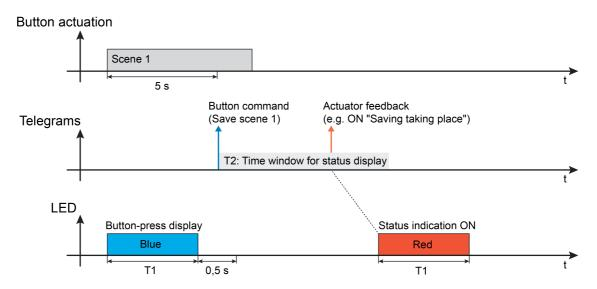
Figure 21: Example of a status display with the operating function "Scene extension" Scene extension with memory function and status display
