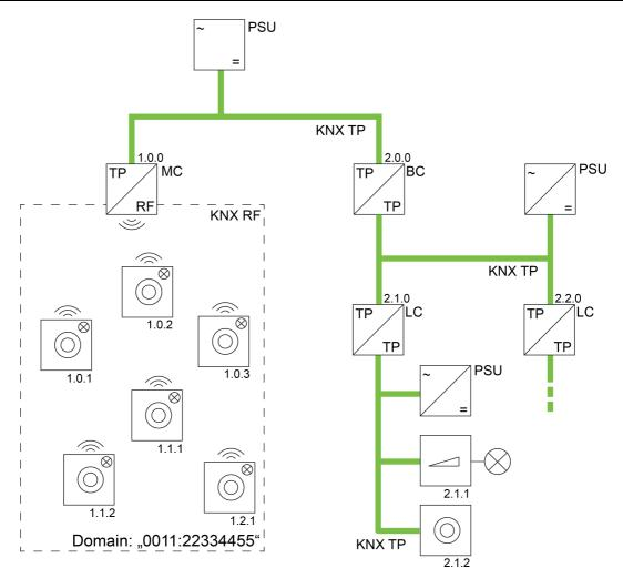
Figure 39: Example of a possible KNX topology with RF and TP lines Media coupler as backbone coupler
