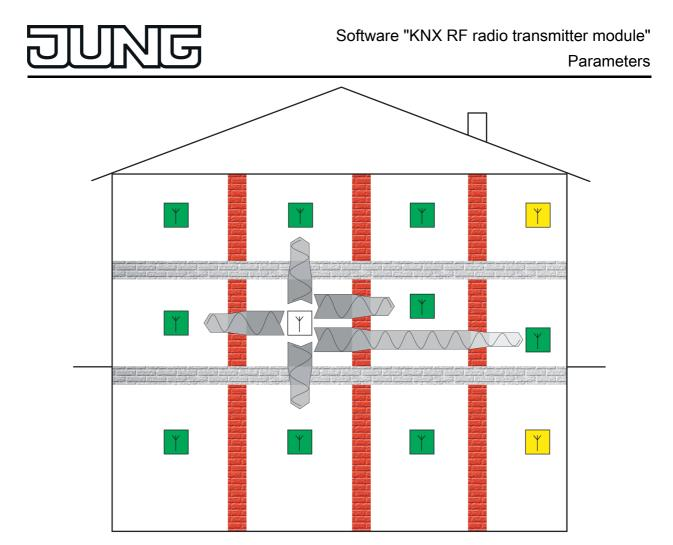
Figure 27: Attenuation of the radio signal in buildings through walls and ceilings Example 2: "Central position of the transmitter" (simplified depiction)
