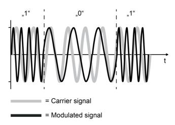
Figure 25: Frequency key shifting as a modulation method (FSK = <u>Frequency Shift Keying</u>)
