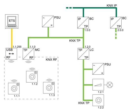
Figure 41: Example of a possible KNX topology with a KNX RF USB data interface
