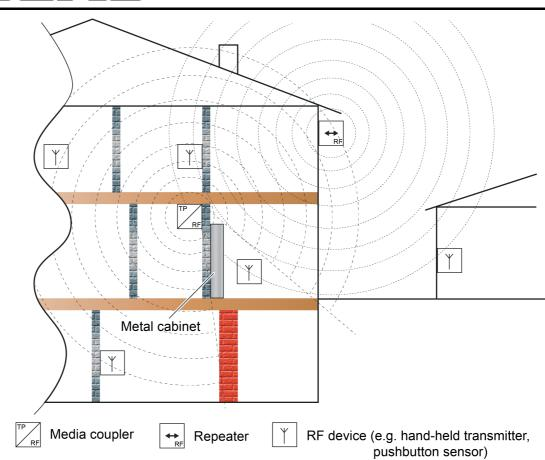
Figure 37: Use of a media coupler as a repeater for signal amplification and elimination of radio shadow for indoor and outdoor applications
