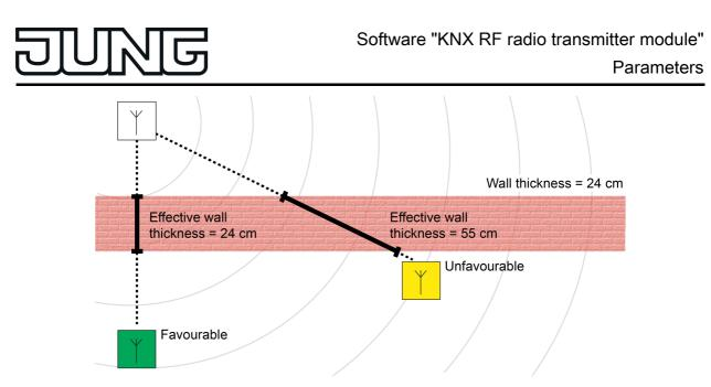
Figure 28: Attenuation through effective wall or ceiling thickness
