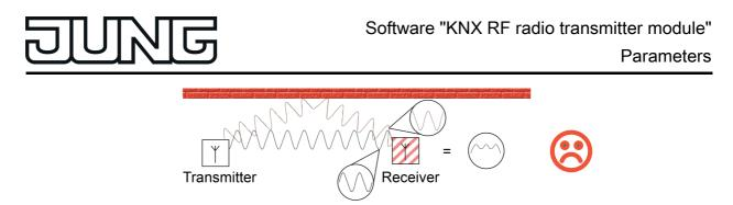
Figure 31: Interference at the receiver prevents reception
