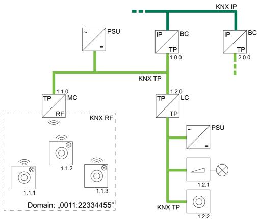
Figure 38: Example of a possible KNX topology with RF, TP and IP lines Media coupler as line coupler
