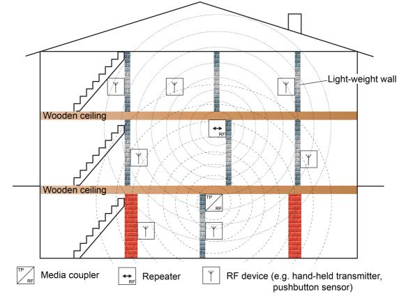
Figure 35: Building structure with one KNX RF line and repeater (example)
