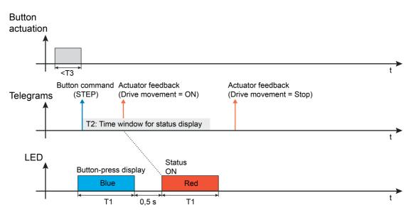
Figure 17: Example of a status display with the operating function "Venetian blind" with a short button-press
