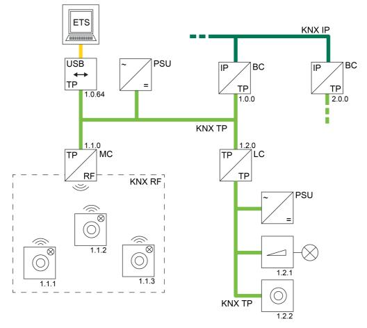
Figure 42: Example of a possible KNX topology with a KNX TP USB data interface
