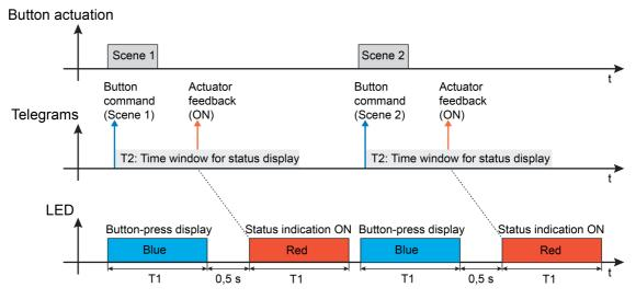
Figure 20: Example of a status display with the operating function "Scene extension" Scene extension without storage function
