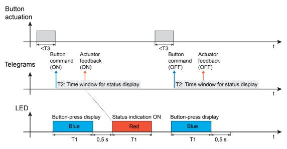
Figure 14: Example of a status display with the operating function "Dimming" with a short button-press
