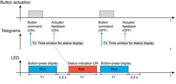
Figure 5: Example of a two-level actuation and status display Status display state "ON" through red LED
