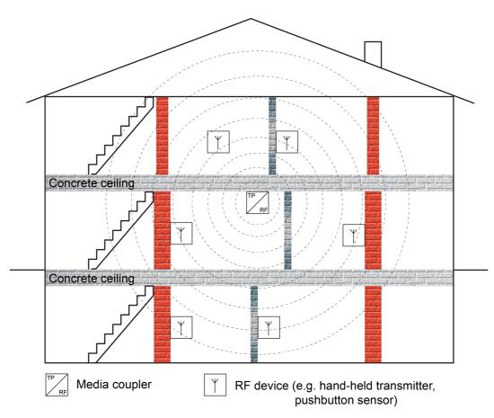
Figure 33: Building with a KNX RF line (example)
