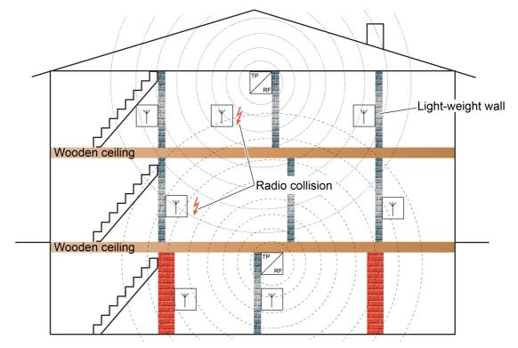
Figure 34: Building structure with two KNX RF lines, disadvantageous influence (example)
