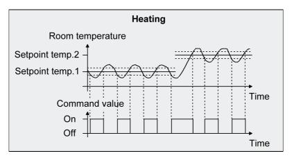
Figure 33: 2-point feedback control for the single "Heating" operating mode
