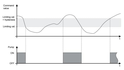
Figure 8: Pump control with sample command value characteristic
