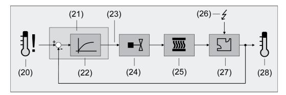
Figure 30: Controlled system of single-room temperature control
