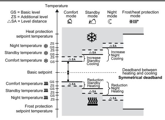
Figure 49: Setpoint temperatures in the operating mode "Basic and additional heating and cooling" with symmetrical deadband
