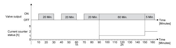
Figure 29: Function of the operating hours counter (using the example of an up-counter)
