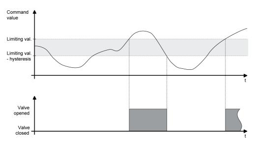
Figure 17: Example of command value evaluation with limiting value
