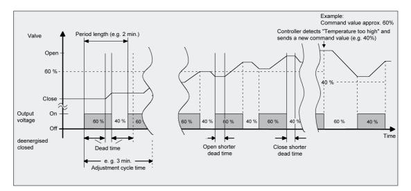
Figure 19: Ideal course of the valve stroke for a cycle time < Adjustment cycle time
