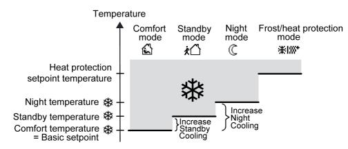
Figure 45: Setpoint temperatures in the operating mode "Cooling"
