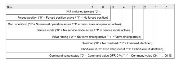
Figure 20: Bit encoding of the object "Feedback combined valve status"
