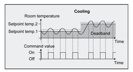
Figure 36: 2-point feedback control for mixed "Heating and cooling" mode with active cooling operation.
