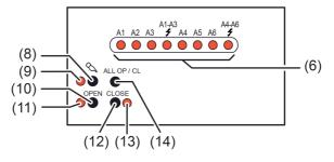
Figure 4: Controls and indicators on the front panel of the device
