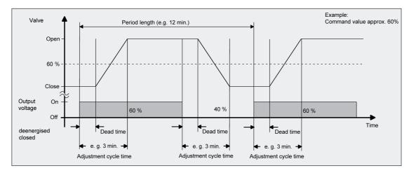
Figure 18: Ideal course of the valve stroke for a cycle time > 2 x Adjustment cycle time
