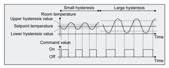
Figure 38: Effects of the hysteresis on the switching behaviour of the command value of 2-point feedback control
