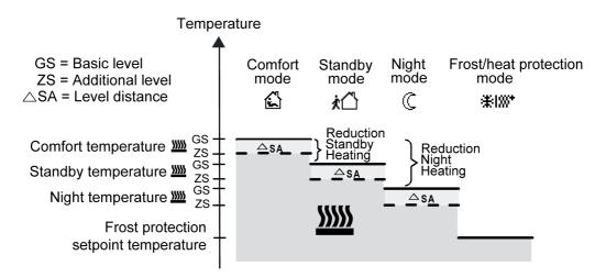
Figure 44: Setpoint temperatures in the operating mode "Basic and additional heating"
