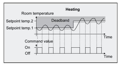
Figure 35: 2-point feedback control for mixed "Heating and cooling" mode with active heating mode.
