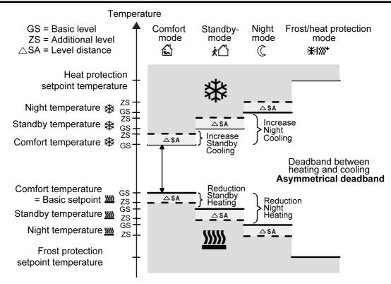
Figure 50: Setpoint temperatures in the operating mode "Basic and additional heating and cooling" with asymmetrical deadband
