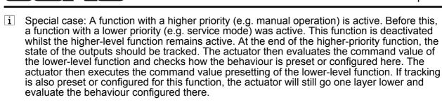
Example 1: Service mode is active (valve completely opened / 100 % command value). A value of 10 % was most recently preset via a command value telegram (normal operation). No other functions are active. Service mode is configured in such a way that the starting state should be <u>tracked</u> at the end of this function.
