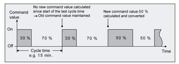
Figure 32: Switching PI control
