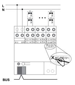
Figure 2: Connection of actuators 230 V
