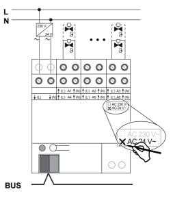
Figure 3: Connection of actuators 24 V
