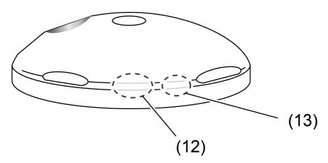
Figure 10: Position of the programming LED and reed contact
