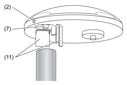
Figure 6: Mounting on freestanding mast without fastening arm
