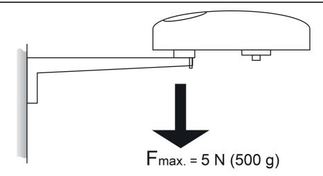
Figure 5: Maximum load on the fastening arm
