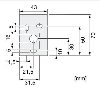
Figure 8: Fastening arm – dimensions for boreholes
