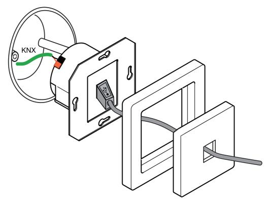
Figure 4: Device connection (FM design)
