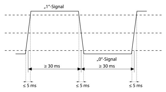
Figure 9: S0 pulse signal waveform
