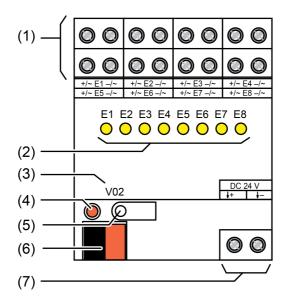
Figure 1: Device components binary input 8-gang 12...48 V
