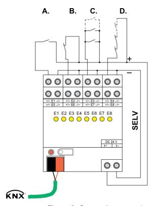
Figure 2: Connection examples Contacts exclusively supplied internally
