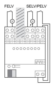
Figure 5: Connection example SELV/PELV and FELV circuits
