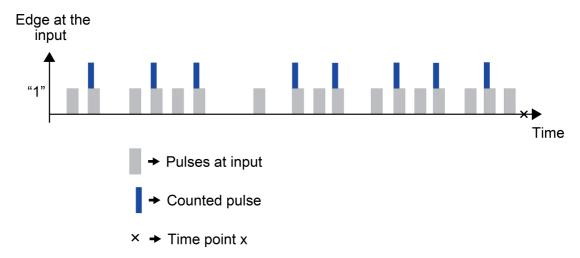
Figure 16: Example for setting the number of changes in counter status per counted pulse
