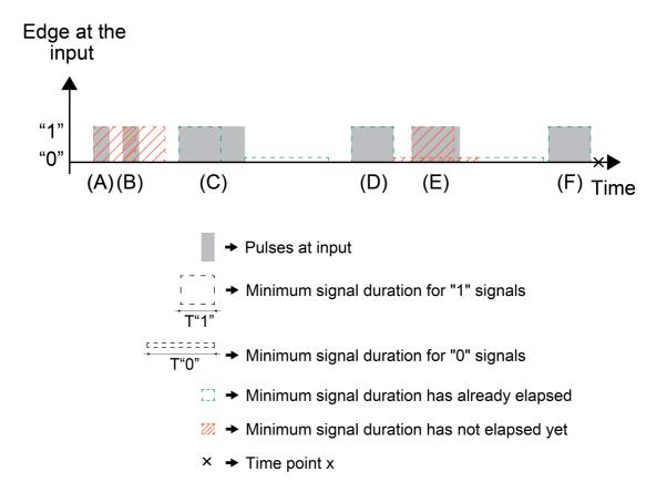
Figure 17: Example for setting the minimum signal duration
