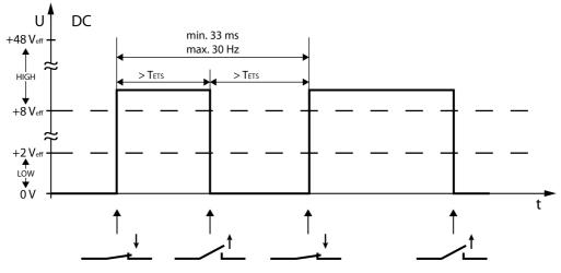
Figure 7: Example for a signal sequence of a direct voltage signal (DC)
