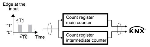
Figure 14: Pulse counter, functional diagram
