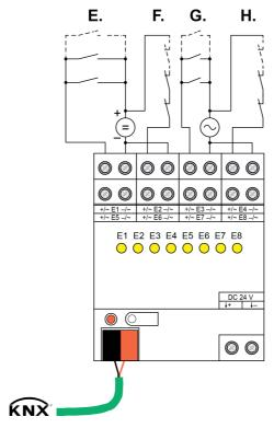
Figure 3: Connection examples Contacts exclusively supplied externally
