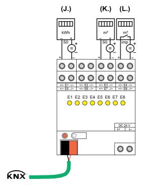
Figure 4: Connection example Connecting the S0 interface
