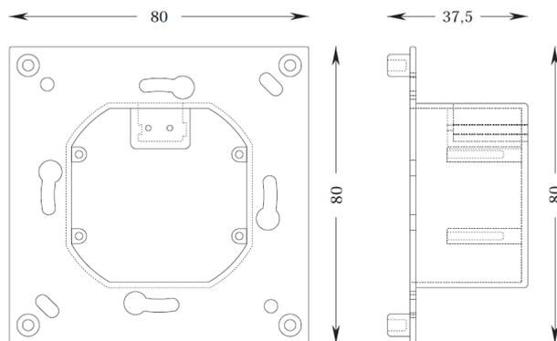
Picture 2: Dimensions of the Installation Box – Bus Coupler
