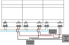
At maximum three power supplies can be connected in parallel.
