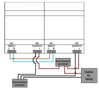
At maximum three power supplies can be connected in parallel.
