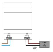
The mains voltage is connected to the left 2-pin screw terminal "AC INPUT".
