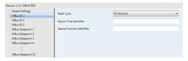
MBus-ID 1 - MBus-ID 3 corresponds to the device connections 1 - 3  $\,$
