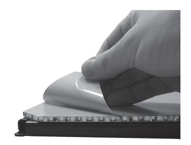
Once the protective carrier layer has been removed from the front panel, position the loudspeaker into the routed area. It is vital that the entire surface area of the speaker's active panel bonds to the routed out area of the board.
