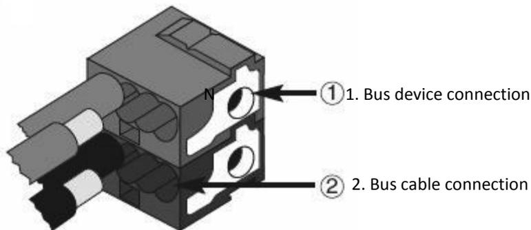
2. Insulate the screen, the electrical continuity conductor and the remaining white and yellow wires of the bus cable (should a bus cable with 4 conductors be used), which are not needed.
